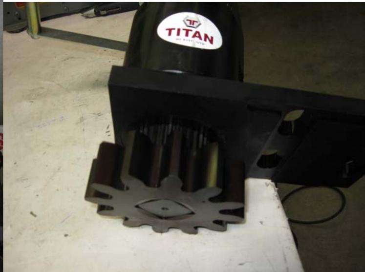
Another SUPERIOR BOLTING SOLUTION® from Titan Technologies. This adaptor converts your Titan Electric Torque Wrench into a tool to **rotate the Hub on wind turbines with the blades attached.**
