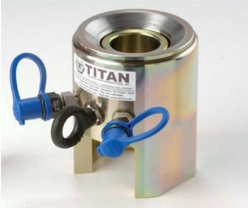
TITAN manufactures standard and custom built tooling for sub sea use. The standard tool range incorporates a combined body and bridge, lifting eye bolt, 30 mm piston stroke, 1500 bar operating pressure, twin hydraulic connections, a maximum piston stroke indicator and a split reaction nut. Lower cost solid reaction nuts are also available. These tools are fitted with the TITAN composite material high pressure seals which clip into place and require no adjustment.
