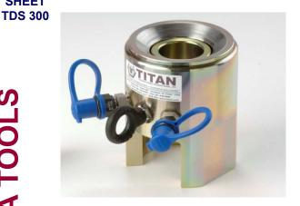
**TITAN** manufactures standard custom built tooling for sub sea use. The standard tool range incorporates a combined body and bridge, lifting eye bolt, 30 mm piston stroke, 1500 bar operating pressure, hydraulic twin connections, a maximum piston stroke indicator and a split reaction nut. Lower cost solid reaction nuts are available. These tools are fitted with the TITAN composite material high pressure seals which clip into place and require no adjustment.
